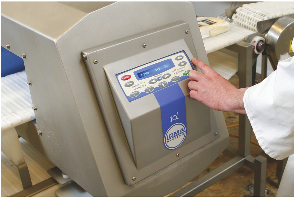
Control panel, above, features a graphics-driven touchscreen that helps simplify communication and operation issues. Right, Alpine Slicing & Cheese's finished packs of cheese exit the IQ3 metal detector and convey to a manual case-packing area.
