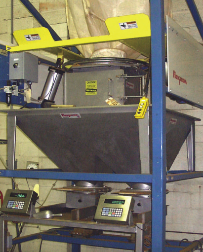
Top, an operator prepares a lined case for filling. The case will be loaded with 50 lb of spices on the feeding/bagging unit, below.
